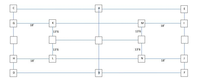
The court is now ready to be lined and should look like the diagram below. The lines should be painted so that the string is on the outside of each line, apart from the centre service line and centre marks where the string should be in the middle of the line. The centre marks each need to be approximately 4 inches long.
