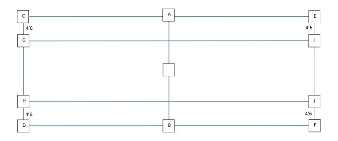
• Measure 18 feet from pegs G, H, I and J along each singles side line and push pegs into the ground. We'll call these pegs K, L, M and N - they mark the service lines. Tie two strings to connect them so they run parallel to the base lines, these are the service lines.
